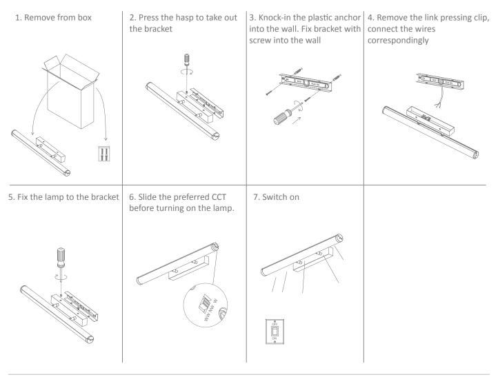
Note: -The lamp must be installed by professional electrician -Ensure the power supply is switched off before fitting this product -Do not touch the lamp when in use -Keep away from hot steam and corrosive gas
